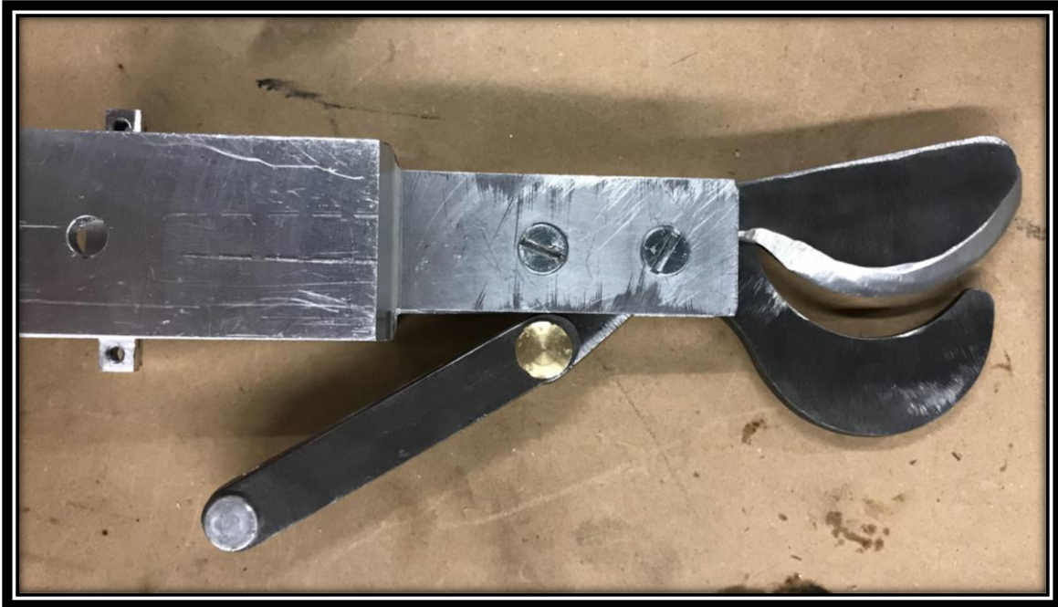
L3: Aluminum blade housing and stainless steel blade.
